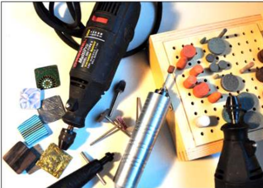
Fig 2.9.14.1 Flex Shaft – Flex Shaft Kit Used for Various Purposes
