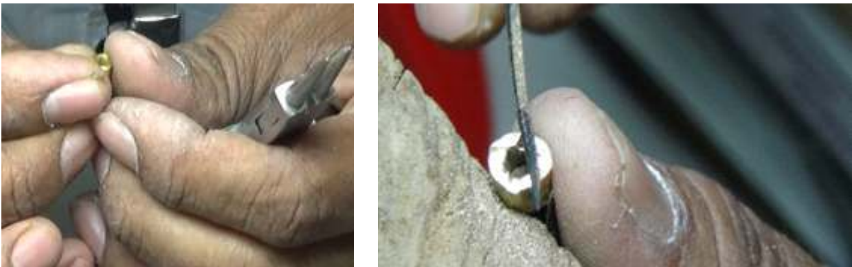
Fig 3.4.1.6 Filing the cavities between the collet prongs
