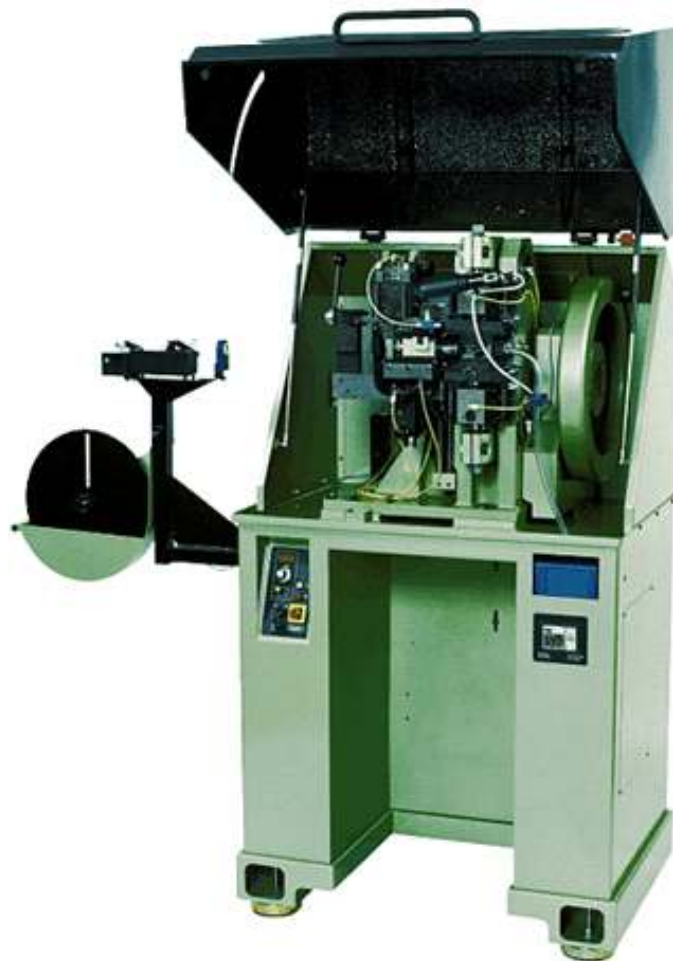
Fig 3.2.8.1 Hollow bead and ball making machine
