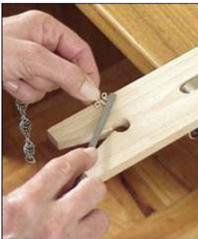
Fig 4.4.4.1 Filing of Soldered Jewellery
