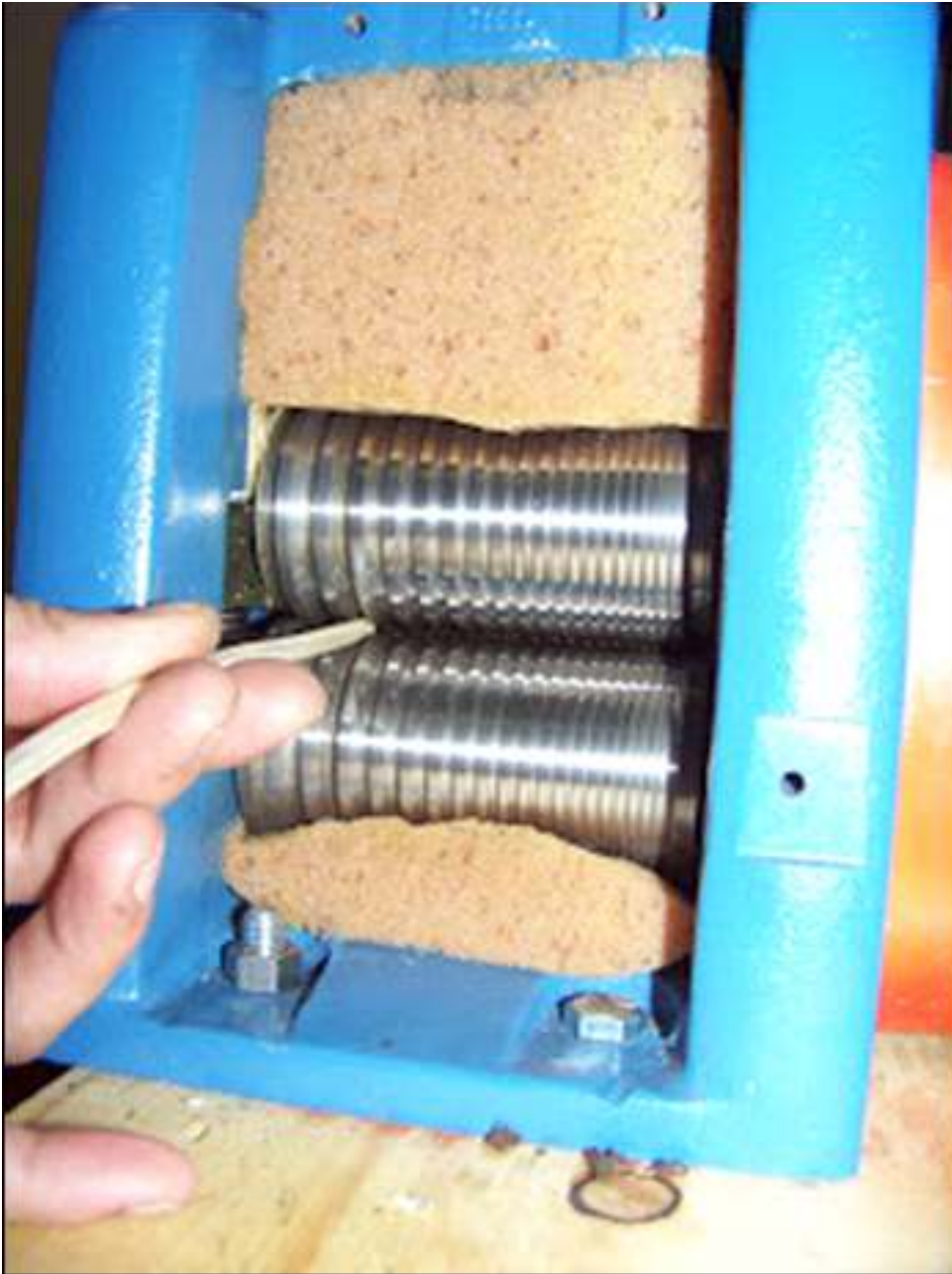
Fig 2.9.2.3 Wire drawing – After annealing put the wire again in the roll mill to make It thinner
