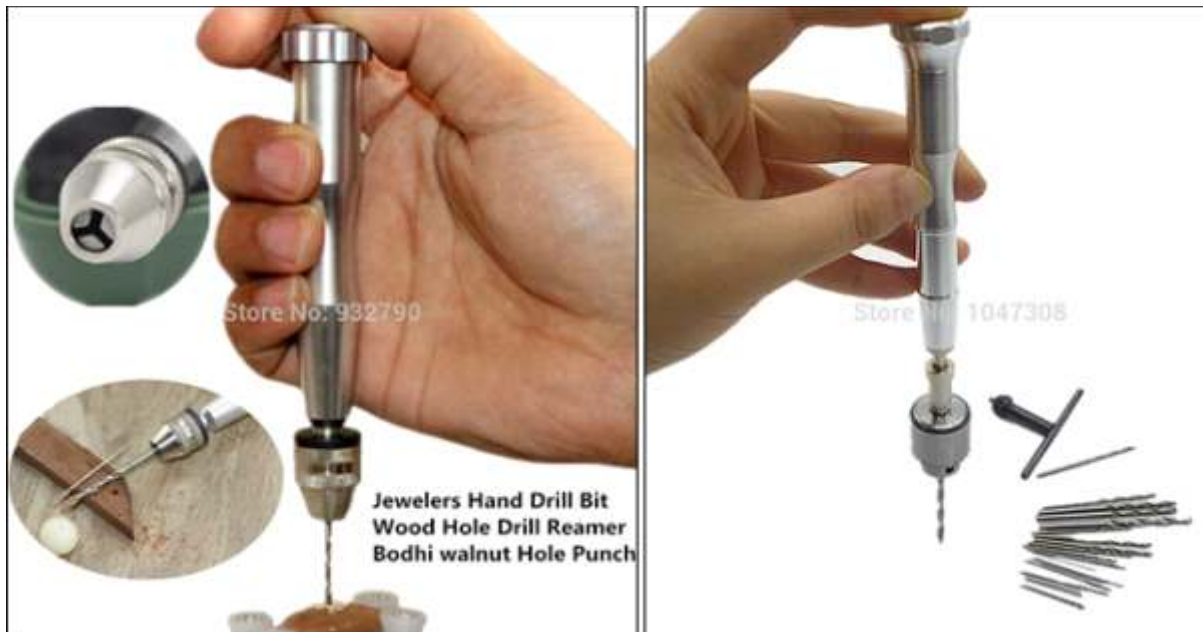
Fig 2.9.19.1 Drilling Tools – Hand Drill and Small Drill Bits Are Used for Drilling Areas for Setting Stones or Links
