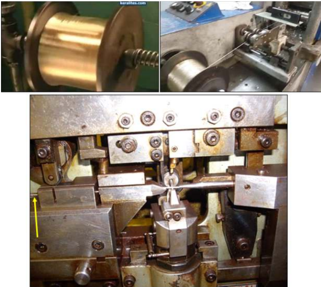
Fig 3.7.4.2 Machine made chains – Top left (coiled wire on spool), Top right (wire being pulled into machine for making wire), bottom (arrow shows the wire going into machine and getting shaped into chain)
