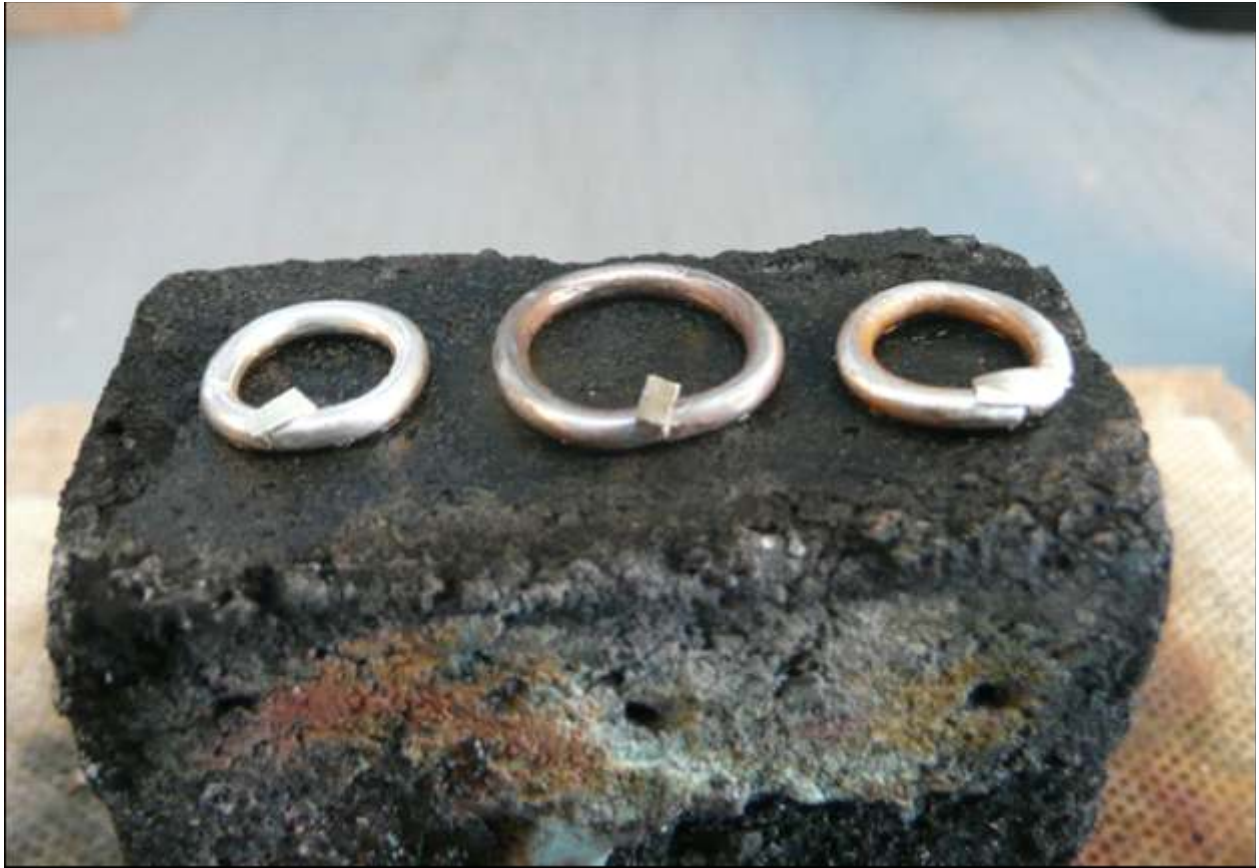
Fig 3.7.10.1 Product defect repairing – shank of ring is uneven and the 3 rd ring requires re-cutting and re-soldering
