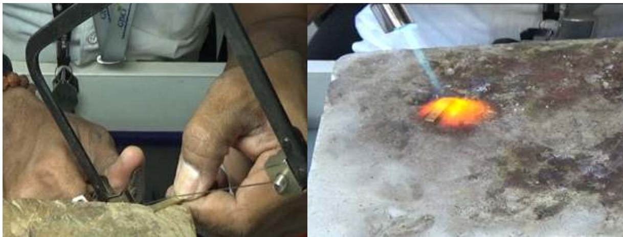
Fig 3.4.1.2 Measured strip cut and annealed
