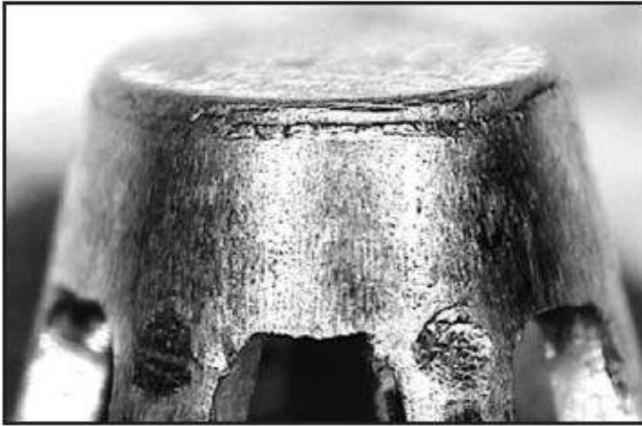
Figure 3 - Failed cup setting
