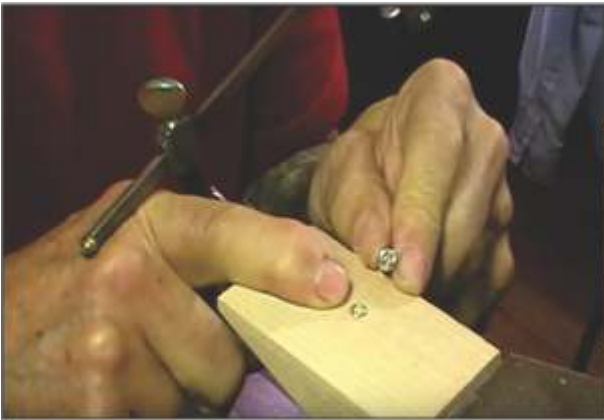
Step 1: Make spiral coil and cut single jump rings
