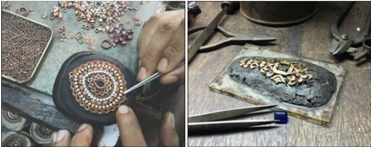
Fig 4.3.6.1 Check the Stone Size with the Setting Frame for the Stones
