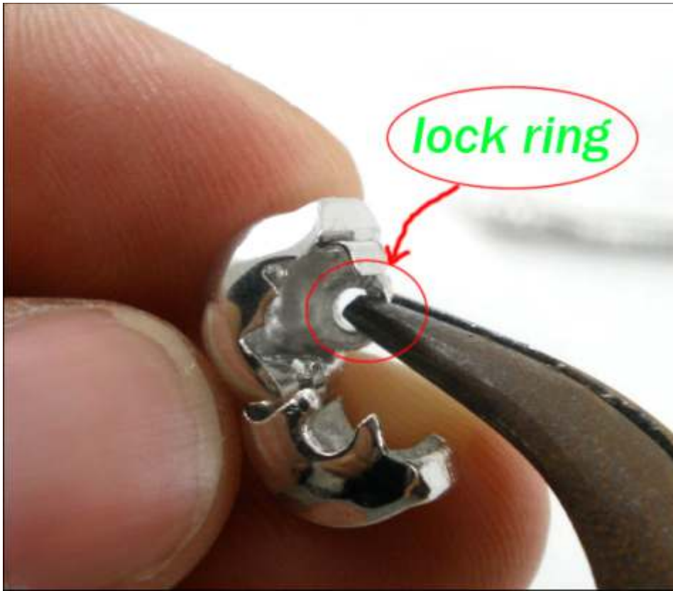
Fig 4.5.1.2 Product Defects – Damaged Component or Finding
