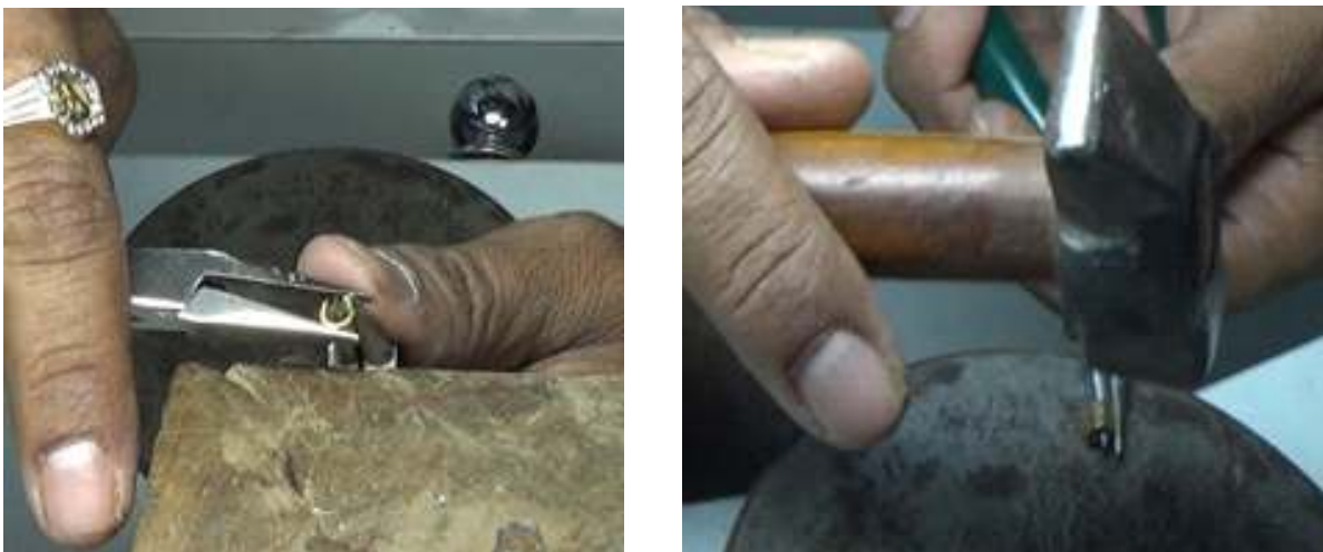
Fig 3.4.1.4 Shaping collet to get round shape
