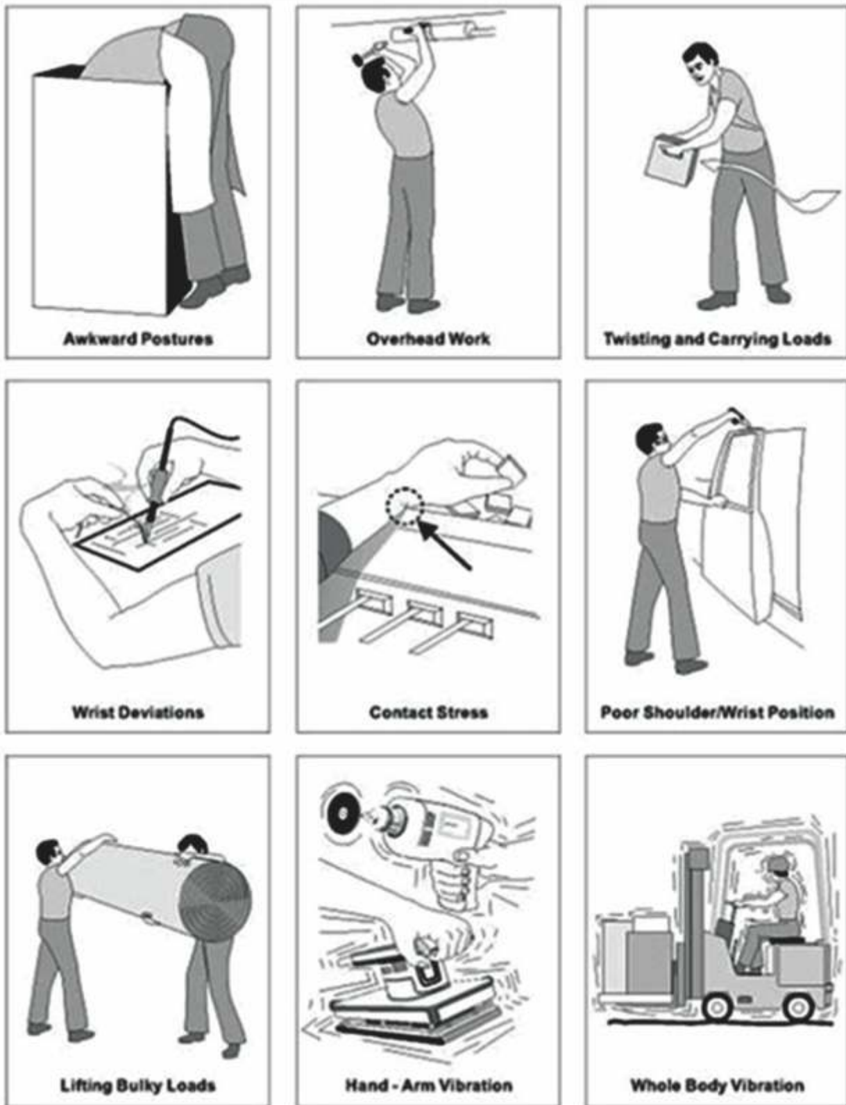
Fig 6.3.1.4 Problems to avoid
