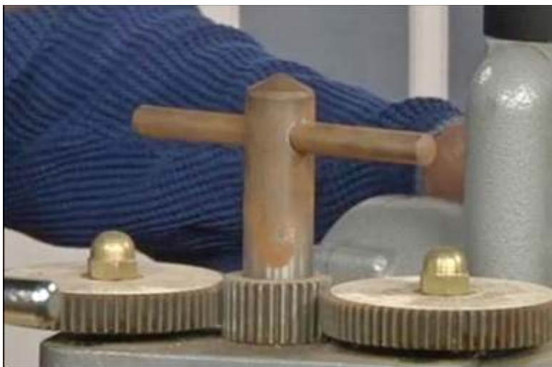
Fig 2.9.1.3 Rolling mill – Adjusting wheels
