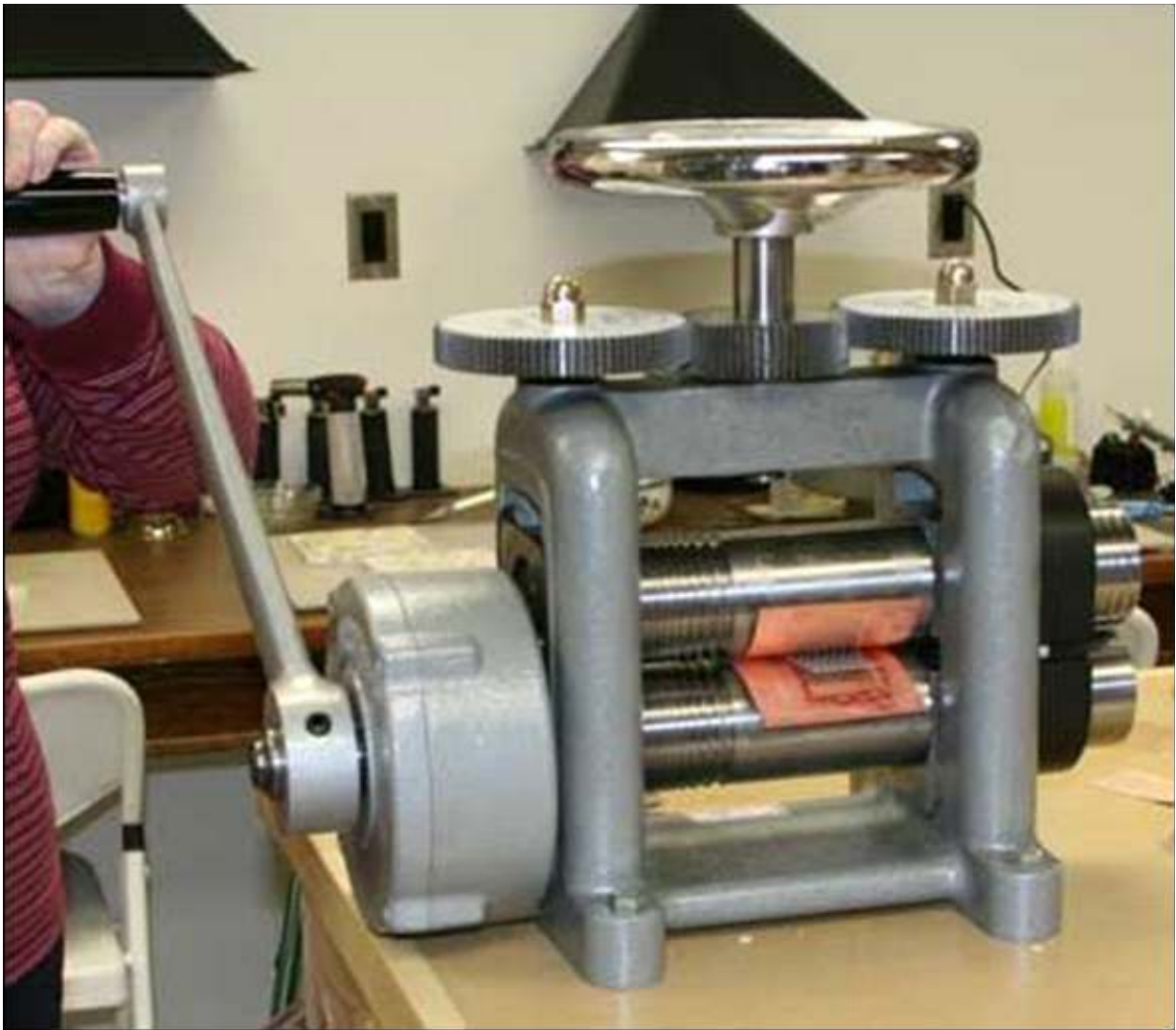
Fig 2.9.1.4 Rolling mill – Metal sheet being adjusted for thickness
