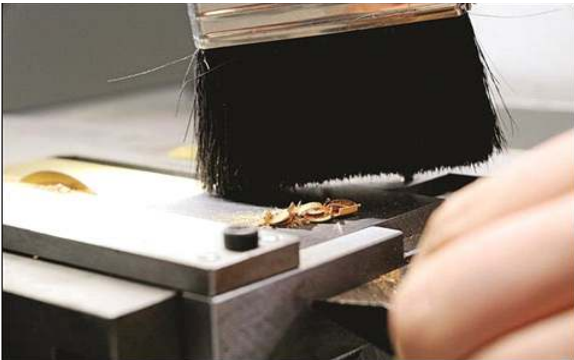
Fig 4.6.1.1 Collecting gold dust and fragments
