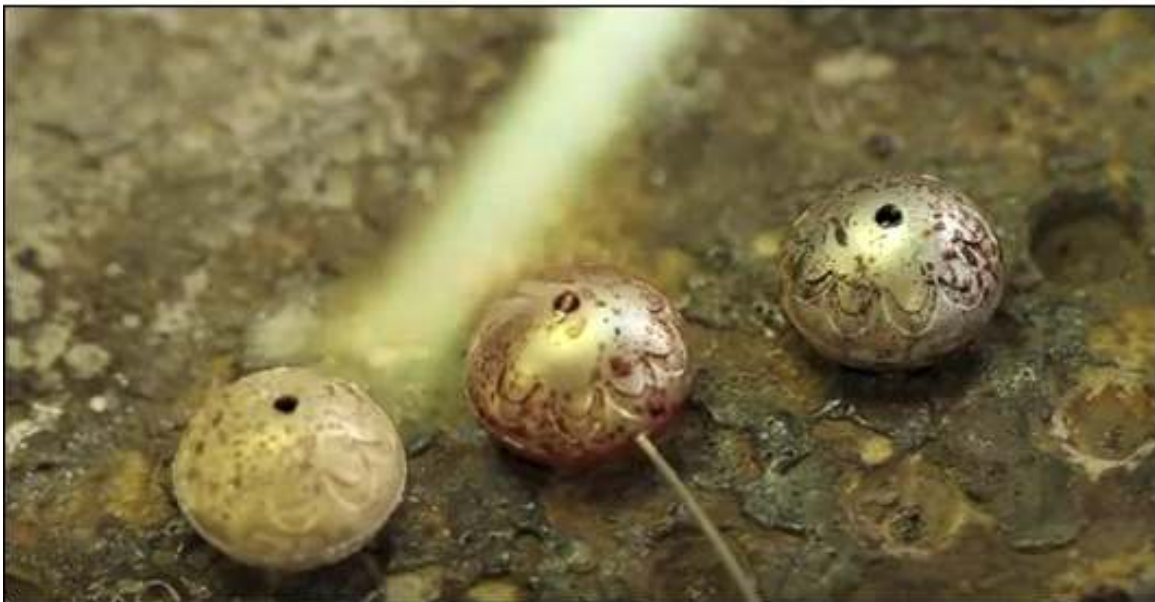
Fig 3.2.5.1 Solder the half spheres
