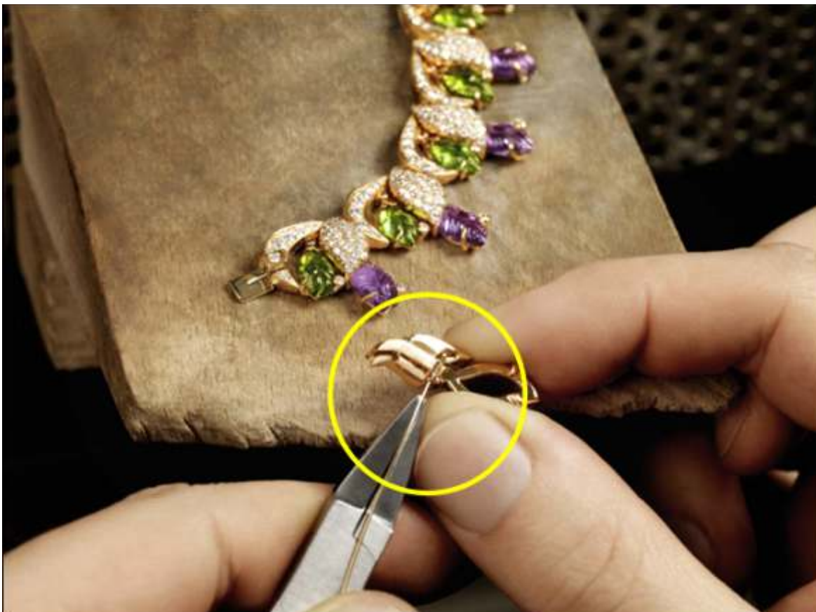
Fig 2.8.1.1 Component being fitted - Hinge
