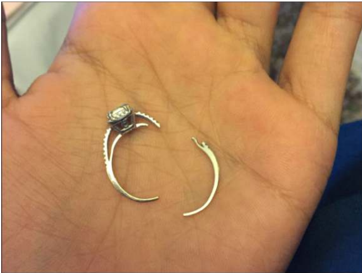
Fig 4.5.1.1 Product Defects – Excessive Filing
