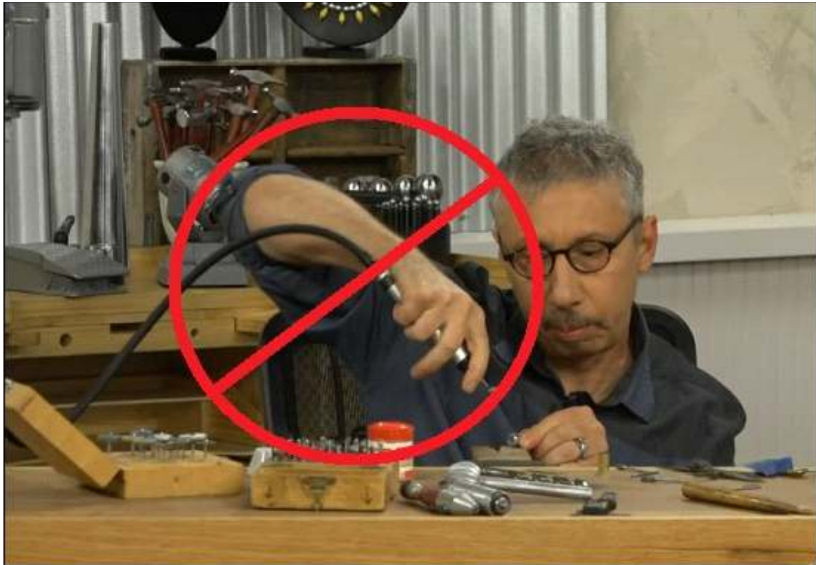
Fig 2.9.14.3 Flex Shaft – Wrong Way of Holding Flex Shaft
