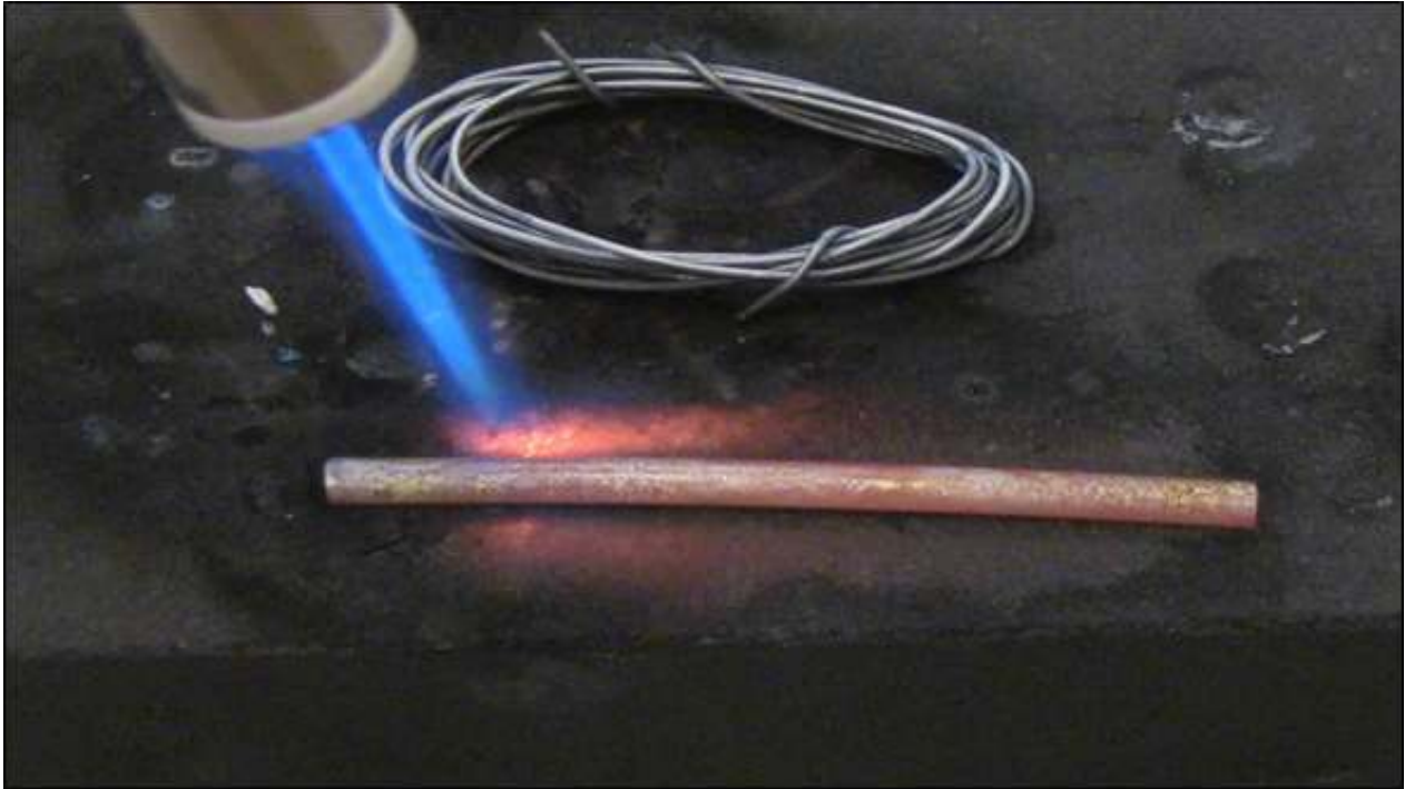
Fig 2.10.2.1 Wire Drawing – Anneal Wire When It Becomes Half the Thickness of Original Thickness
