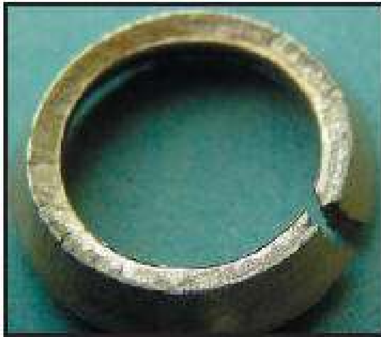
Figure 9 - Fractured ring blank
