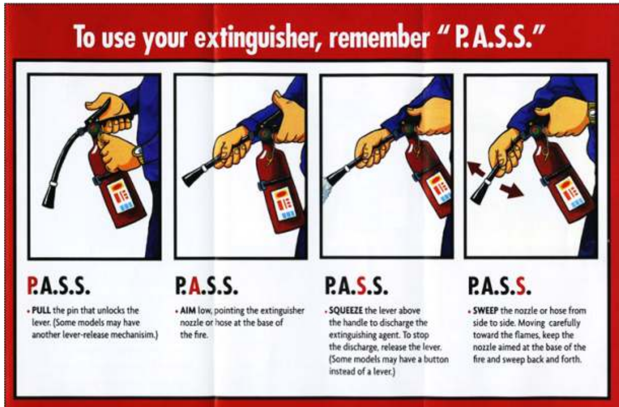
Fig 6.4.2.1 Steps to use the fire extinguisher – use the right extinguisher for the fire
