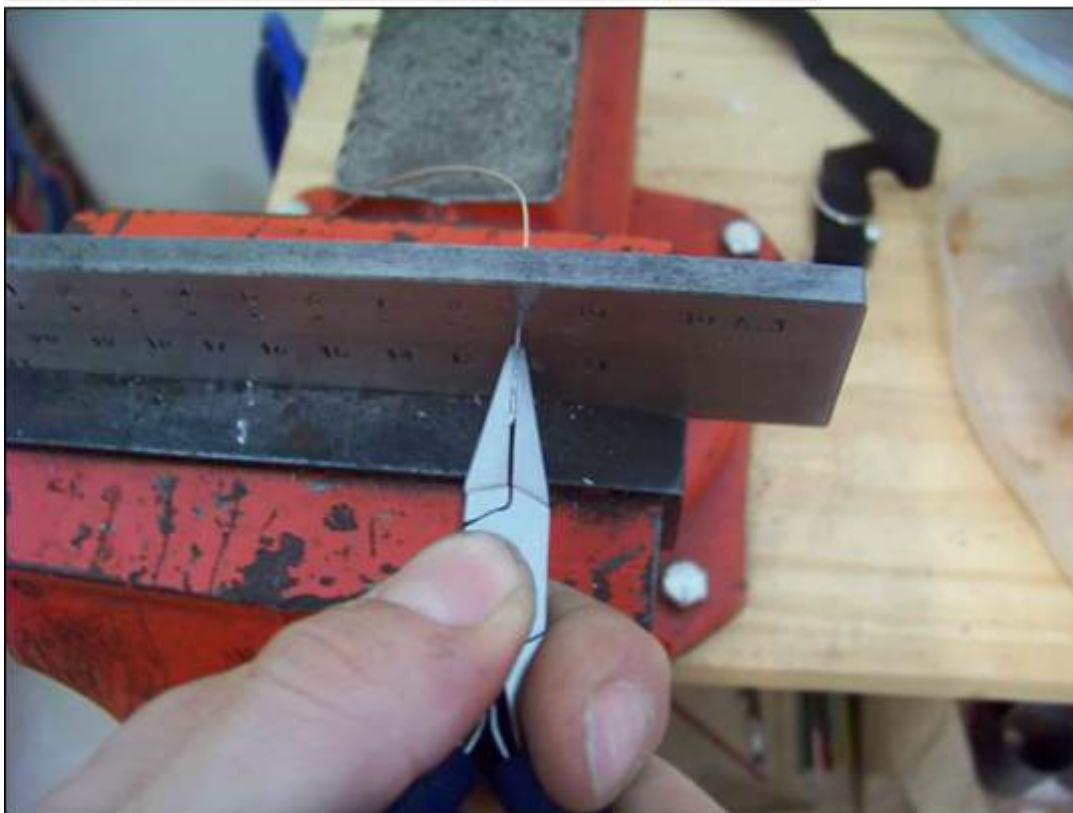
Fig 2.10.4.2 Wire Drawing – First Use the Large Gauge and Move to the Thinnest Gauge, Pull Using the Draw Tong
