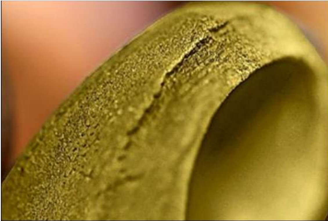
Fig 4.5.1.3 Product Defects – Crack on Ring Shank Due to Annealing Problem During Wire Drawing Process
