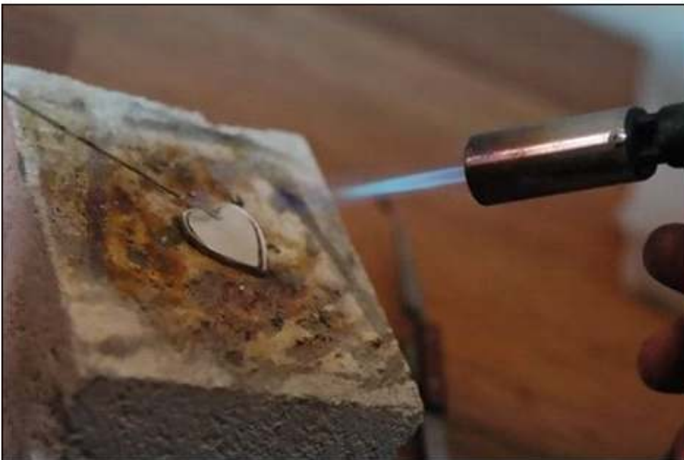
Fig 4.4.1.2 Soldering Wire and Sheet Frames
