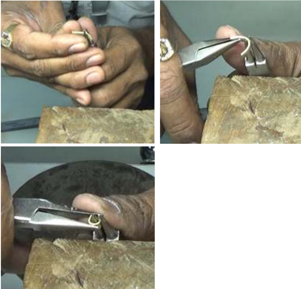
Fig 3.4.1.3 Bending strip using flat plier
