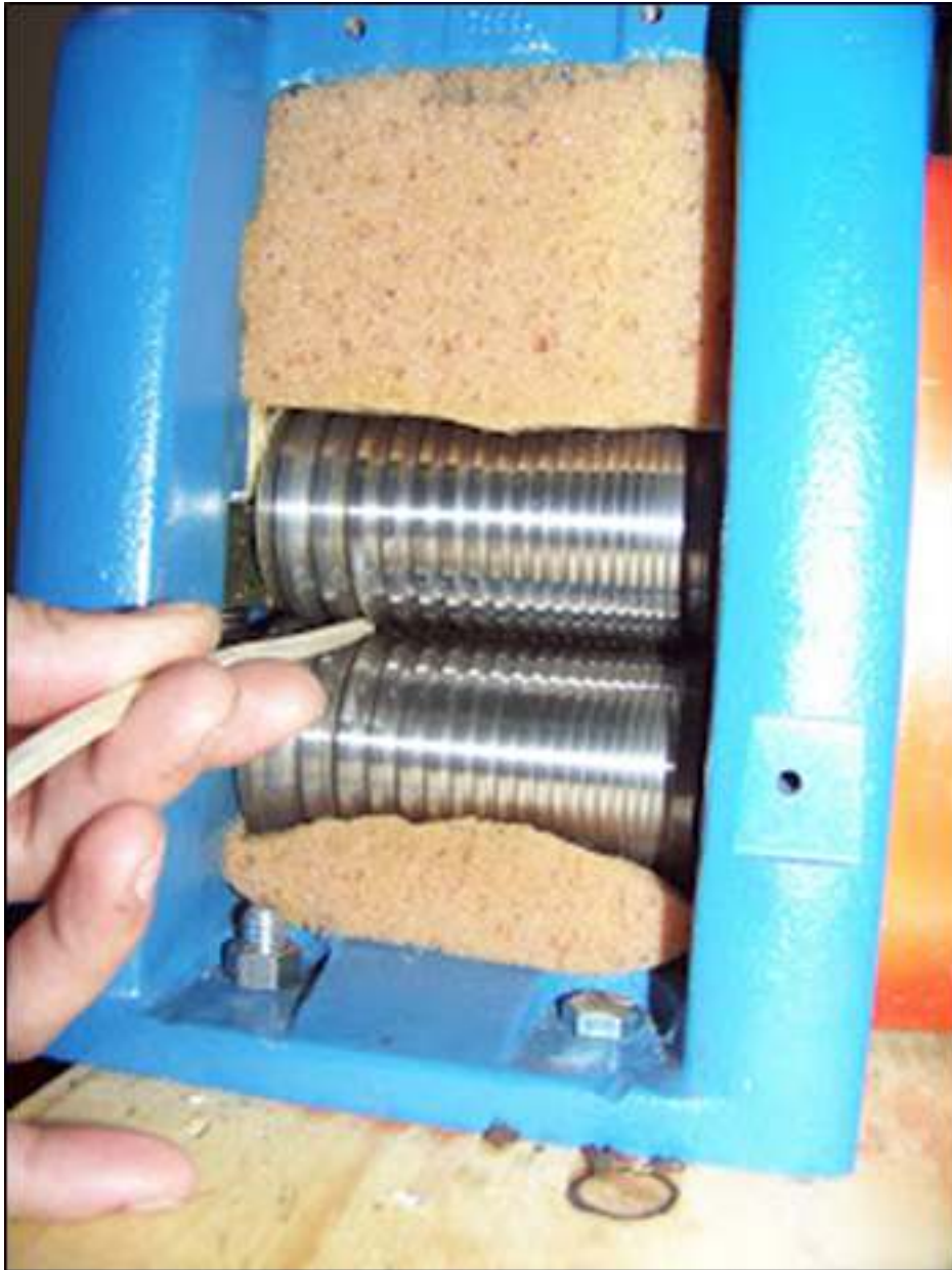
Fig 2.10.3.1 Wire Drawing – After Annealing Put the Wire Again in the Roll Mill to Make It Thinner
