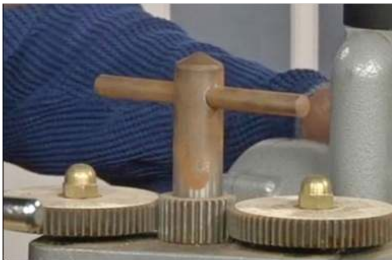
Fig 2.11.1.2 Rolling mill – Adjusting wheels
