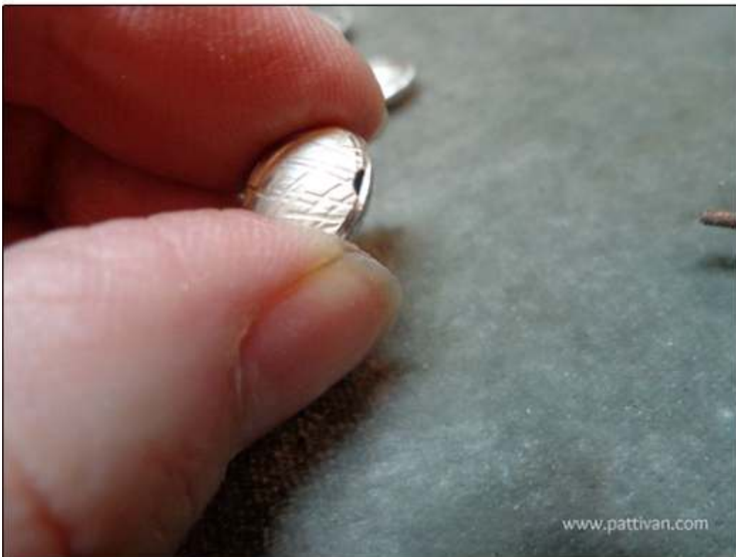
Fig 3.7.9.5 Product defects – metal chipped off during bead making process due to excess hammering
