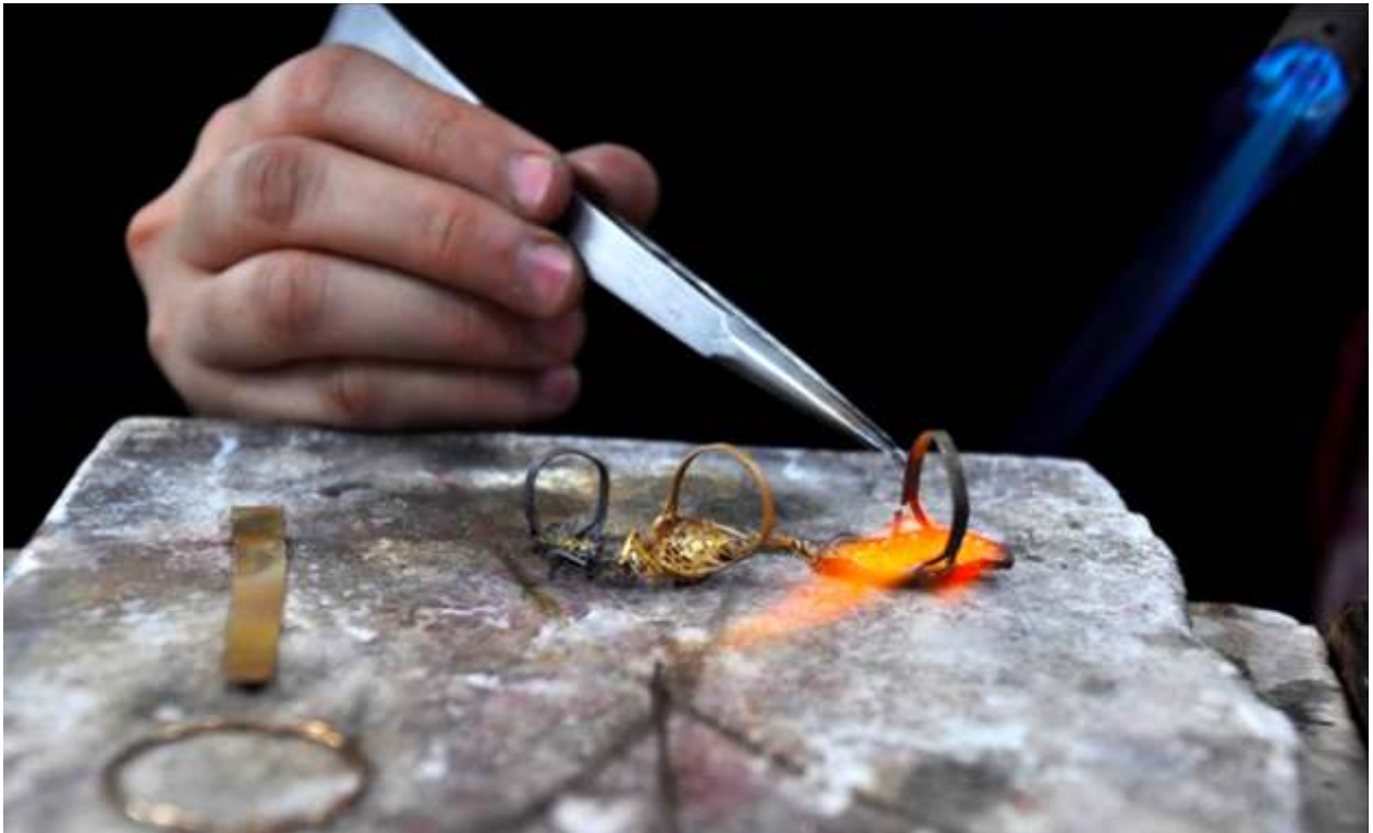
Fig 4.5.2.1 Product Defect Repairing – Shank of Ring is Too Thin and Needs to be Repaired
