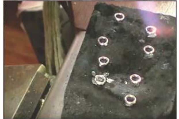
Step 2: Join the ends of the jump rings and keep equal amount of open jump rings
