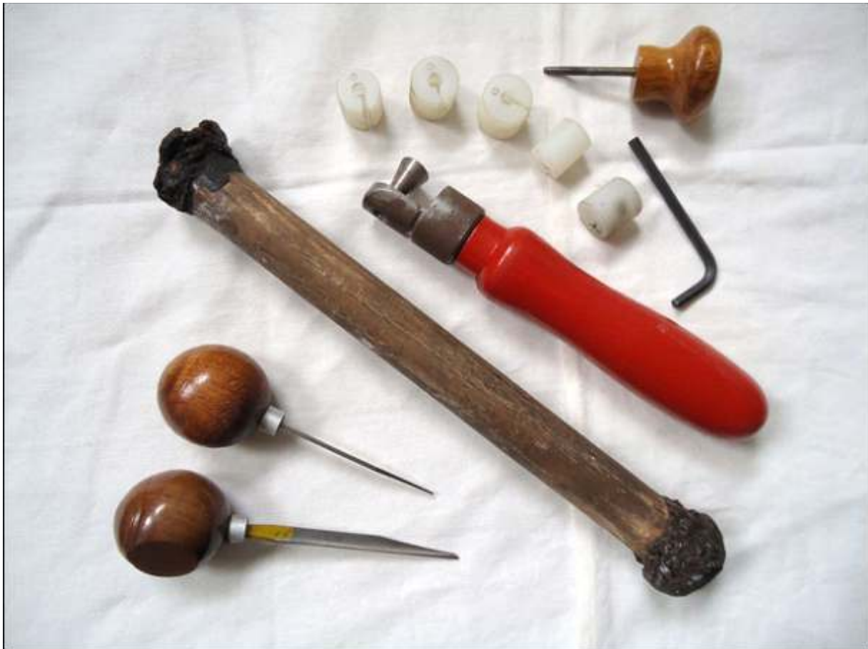
Fig 2.9.7.1 Stone Setting Tools – Prong Pusher, Burnisher, Bezel Roller, Lac Stick
