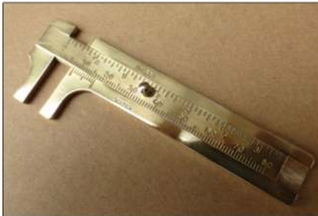
Fig 2.9.16.1 Callipers or Measuring Gauges – Used for Measuring Metal Thickness, Length and Stone Dimensions - 1
