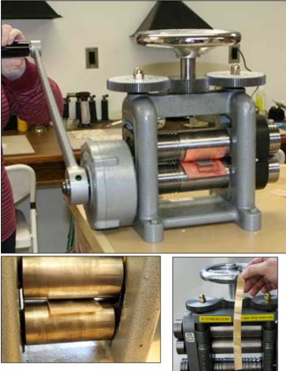
Fig 2.11.2.1 Rolling mill – Metal sheet being adjusted for thickness
